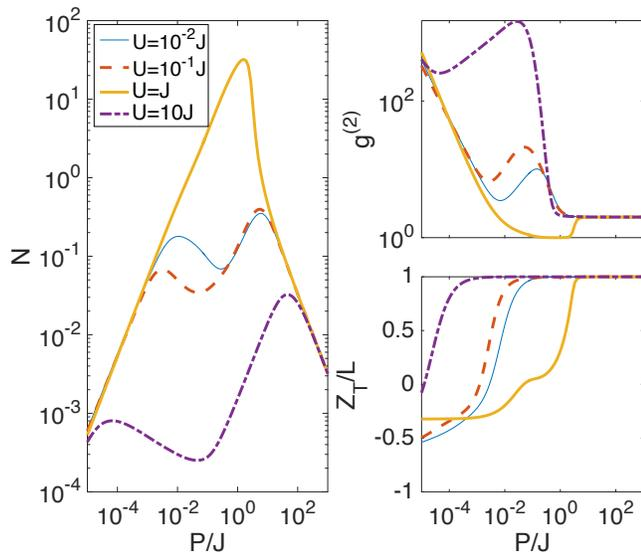
FIG. 2: Cavity photon number (left panel), second order correlation at zero time delay of the emitted radiation (top right panel), and the Z-component of the total atomic spin ( $Z_T$ ) divided by the number of atoms, for the case with  $L = 4$  emitters (bottom right panel), as a function of the external pump and for different values of the interaction energy. The model parameters assumed in the calculations are  $g = 0.1J$  and  $\kappa = 0.5g$ , respectively.
