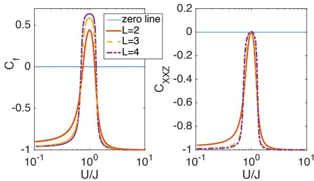
FIG. 4: Cooperativity of the manybody laser as compared to single emitter-lasers (left panel), as defined in Eq. (6). Cooperativity of the manybody laser as compared to the corresponding standard laser (right panel), as defined in Eq. (7). The system parameters used in these simulations are  $g = 0.1J$ ,  $\kappa = 0.5g$ , and  $P = J$ .
