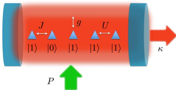
FIG. 1: Pictorial representation of the laser with a strongly interacting manybody system of emitters as the active medium. The microscopic energetic contributions of each possible interacting process are explicitly indicated.
