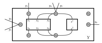
There are two input boxes  $X_1 = \{x_1, ..., x_6\}$  and  $X_2 = \{x^1, x^2\}$ , an output box  $Y = \{y_1, ..., y_6\}$ , and seven cables  $\{c_1, ..., c_7\}$ . In general, there can be any finite numbers of input boxes and cables, and each input/output box is a finite set. For each element z in the input boxes and the output box, we need to specify a cable c to which z is connected. For instance,  $x_4$ ,  $x_5$ , and  $x^2$  are connected to the cable  $c_6$ .
