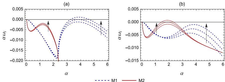
FIGURE 4. Two instability modes M1 and M2 manifest as short wave instabilities beyond a critical Marangoni number. (a) Mode M1 becomes unstable;  $Ca = 10$ ,  $Ma = 11631.21$ , 12231.21, 12831.21. (b) Mode M2 becomes unstable;  $Ca = 100$ ,  $Ma = 9932.65$ , 10832.65, 11732.65. Other parameter values:  $m = 1.5$ ,  $n = 1$ ,  $D_r = 0.5$ ,  $K = 0.5$ ,  $Pe = 2000$ ,  $\gamma = 0.5$ . The arrow indicates the direction of increasing  $Ma$ .
