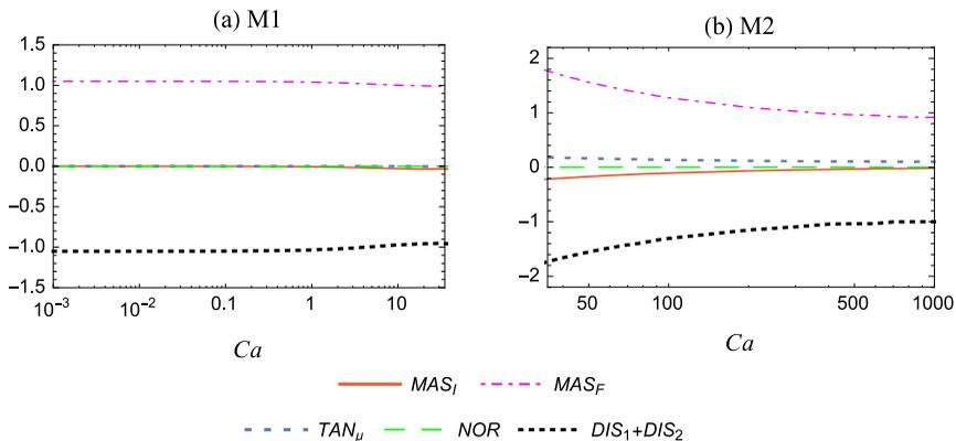
FIGURE 8. Energy budget of the critical M1 and M2 short wave modes plotted in Fig. 6 and Fig. 10b as a function of  $Ca$ . The  $REY_i$  terms are identically zero because  $Re = 0$ . Parameter values:  $n = 1$ ,  $m = 1.5$ ,  $D_r = 0.5$ ,  $K = 0.5$ ,  $Pe = 2000$ ,  $\gamma = 0.5$ .
