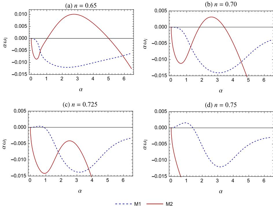
FIGURE 12. Transition from a short wave to long wave instability as  $n$  is increased beyond  $\sqrt{m}$ . Parameter values:  $m = 0.5$ ,  $Ca = 1000$ ,  $Ma = 5000$ ,  $Dr = 1$ ,  $K = 1$ ,  $Pe = 2000$ ,  $\gamma = 0$ .
