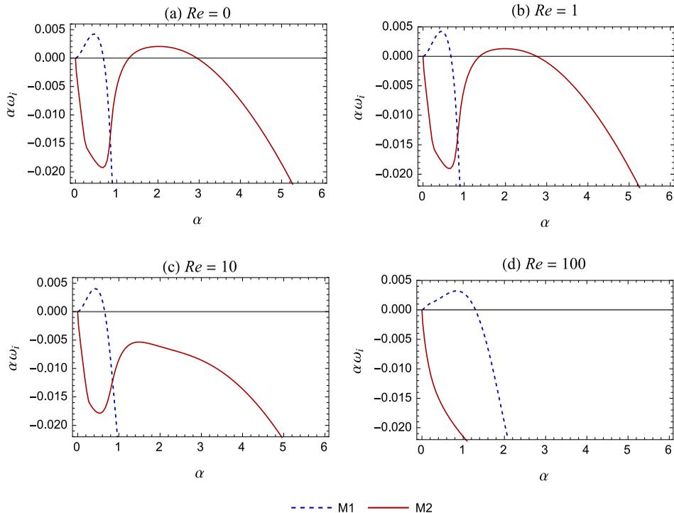
FIGURE 16. Effect of inertia on the solutal Marangoni instability when the M1 mode is long wave. Parameter values:  $Ma = 10000$ ,  $m = 0.9$ ,  $n = 1.3$ ,  $Ca = 1$ ,  $D_r = 0.5$ ,  $K = 1.2$ ,  $\gamma = 0$ ,  $Pe = 1000$ .
