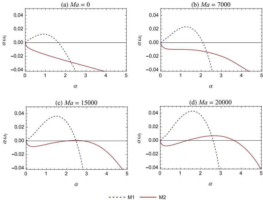
FIGURE 18. Effect of soluble surfactant on the viscosity-induced interfacial instability. The chosen parameter values correspond to the case of  $n^2 > m$ , for which the long wave M1 and short wave M2-SW instabilities are prevalent in the creeping flow limit. Parameter values:  $Re = 100$ ,  $m = 0.5$ ,  $n = 1.3$ ,  $Ca = 1$ ,  $D_r = 0.5$ ,  $K = 1.2$ ,  $\gamma = 0$ ,  $Pe = 1000$ .
