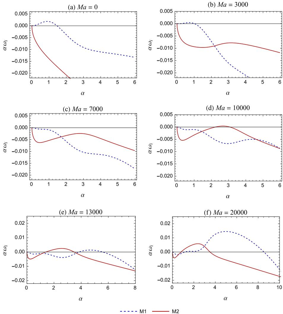
FIGURE 17. Effect of soluble surfactant on the viscosity-induced interfacial instability. The chosen parameter values correspond to the case of  $n^2 < m$ , for which the short wave M1-SW and M2-SW modes are unstable in the creeping flow limit. Parameter values:  $Re = 10$ ,  $m = 1.5$ ,  $n = 1$ ,  $Ca = 100$ ,  $D_r = 0.5$ ,  $K = 1.2$ ,  $\gamma = 0$ ,  $Pe = 2000$ .
