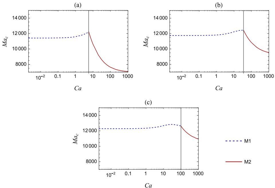
FIGURE 10. Effect of  $Pe$  on mode-switching between short wave M1 and M2 modes. (a)  $Pe = 1000$  (b)  $Pe = 2000$  (c)  $Pe = 2500$  Parameter values:  $n = 1$ ,  $m = 1.5$ ,  $D_r = 0.5$ ,  $K = 0.5$ ,  $Pe = 2000$ ,  $\gamma = 0.5$ .
