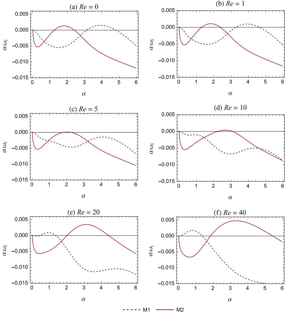
FIGURE 15. Effect of inertia on the solutal Marangoni instability when the M1 mode is short wave. Parameter values:  $Ma = 10000$ ,  $m = 1.5$ ,  $n = 1$ ,  $Ca = 100$ ,  $Dr = 0.5$ ,  $K = 1.2$ ,  $\gamma = 0$ ,  $Pe = 2000$ .
