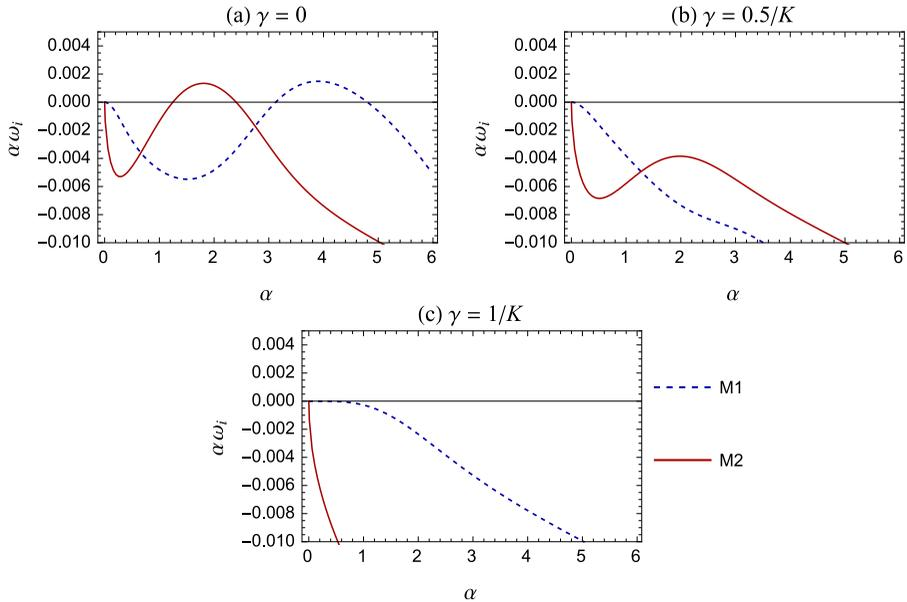
FIGURE 13. Effect of the inter-fluid flux on the short wave instability. Both M1 and M2 short waves are stabilized as the difference of the concentration at the walls from equilibrium is decreased.  $\gamma = 1/K$  corresponds to a base state without inter-fluid flux, as the fluids are in equilibrium in this case and have non-varying concentration profiles. Parameter values:  $m = 1.5$ ,  $n = 1$ ,  $Ca = 100$ ,  $Ma = 10000$ ,  $Dr = 0.5$ ,  $K = 1.2$ ,  $Pe = 2000$ .
