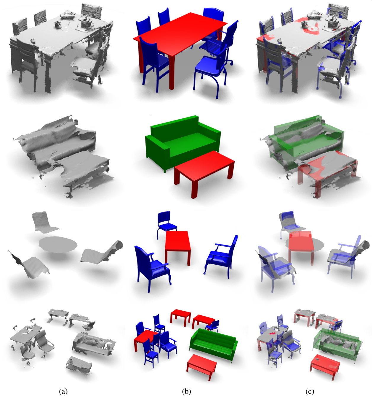
Figure 6: ASIST using a Kinect sensor. Column (a) scanned scene; (b) ASISTs' result; (c) overlay of the previous two.
