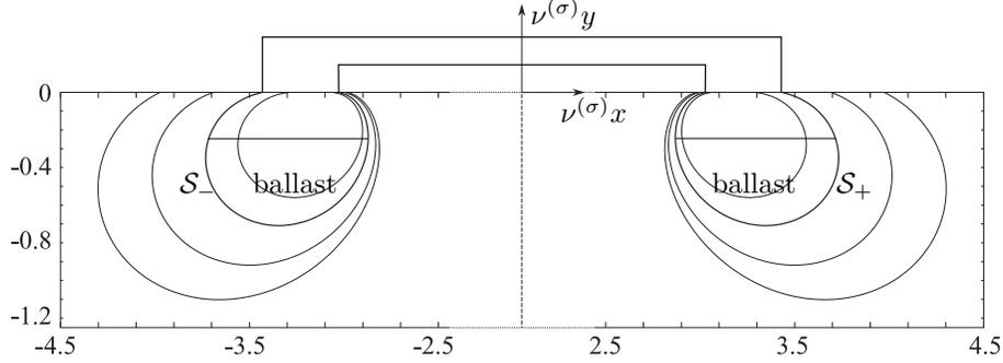
Figure 2: Level lines of the stream function  $\psi_0$  plotted in non-dimensional coordinates. An example of the wetted contours bounding a motionless trapping body is shown in bold and denoted by  $\mathcal{S}_-$  and  $\mathcal{S}_+$ ; other pairs of symmetric streamlines can also be considered as boundaries of immersed parts of trapping bodies. In order to contract the width of the figure, a reduced horizontal scale is applied on the interval  $(-2.5, 2.5)$ .
