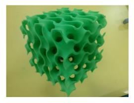
"Gyroid structure" for photonic crystals (*image by* @scifablab).
