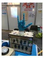
"Hands(H)ome": Prototype of home automation user interface for monitoring and control designed for elders and impaired people (*image by* (*a*)scifablab).
