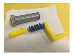
Moineau+Auger pump for volumetric flow proportional to the rotation rate (image by @scifablab)
