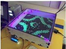
Chladni figures, with the peculiarity of replacing sand with larger spheres moving on a 3D printed net of different geometries and under frequencies adjusted via an Arduino (image by M. Goina @ictpnews)
