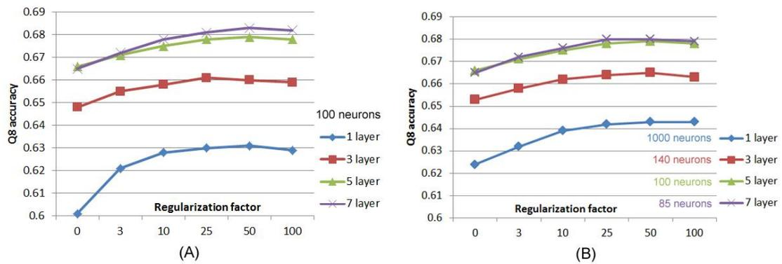
**Figure 4.** The Q8 accuracy on CB513 by the models of different number of layers of 1, 3, 5, and 7 (the same window size is used). (A) Each layer of the 4 models has 100 neurons for a position. The total parameter number of the 4 models is different. (B) Each layer of the models has different neurons for a position. The total parameter number of the 4 models is similar.
