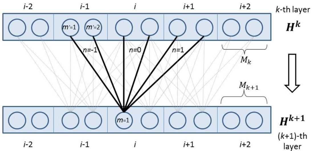
**Figure 6.** The feed-forward connection between two adjacent layers in the deep convolutional neural network.
