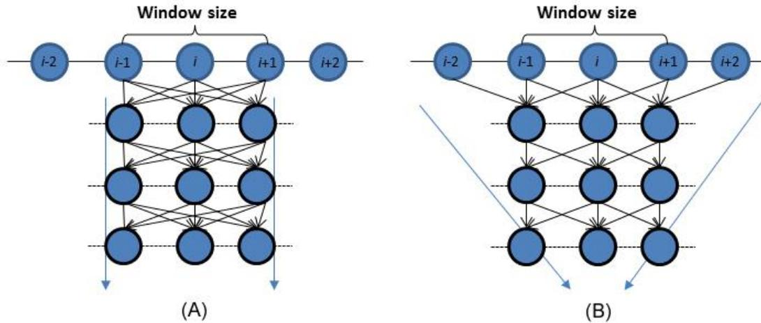
**Figure 1.** A typical deep neural network (A) vs. a convolutional deep neural network (B). A convolutional deep neural network can capture longer-range sequence information than a typical deep neural network when both use the same window size.
