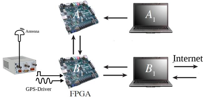
Fig. 6.1: Experimental setup at Location 1 where  $A_1$  and  $B_1$  represent Alice<sub>1</sub> and Bob<sub>1</sub>, respectively. Figure reproduced with permission from Tommaso Lunghi.
