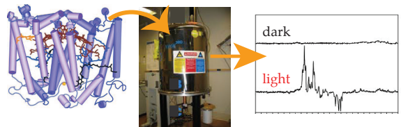
FIG. 10. Schematic of a solid-state photo-CIDNP experiment (the NMR signal was taken from http://ssnmr.lic.leidenuniv.nl/files/ssnmr/10-03.Matysik%20CIDNP.pdf ). A solid sample of reaction centers is placed in a high-field NMR magnet. Upon illumination, an NMR signal is observed, enhanced by several orders of magnitude above thermal equilibrium.
