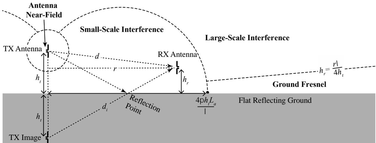
**Figure 1: Cross-section of two-ray propagation from a transmitter to a receiver, separated by a distance  $r$  that may place it in one of several distinct propagation regimes.**
