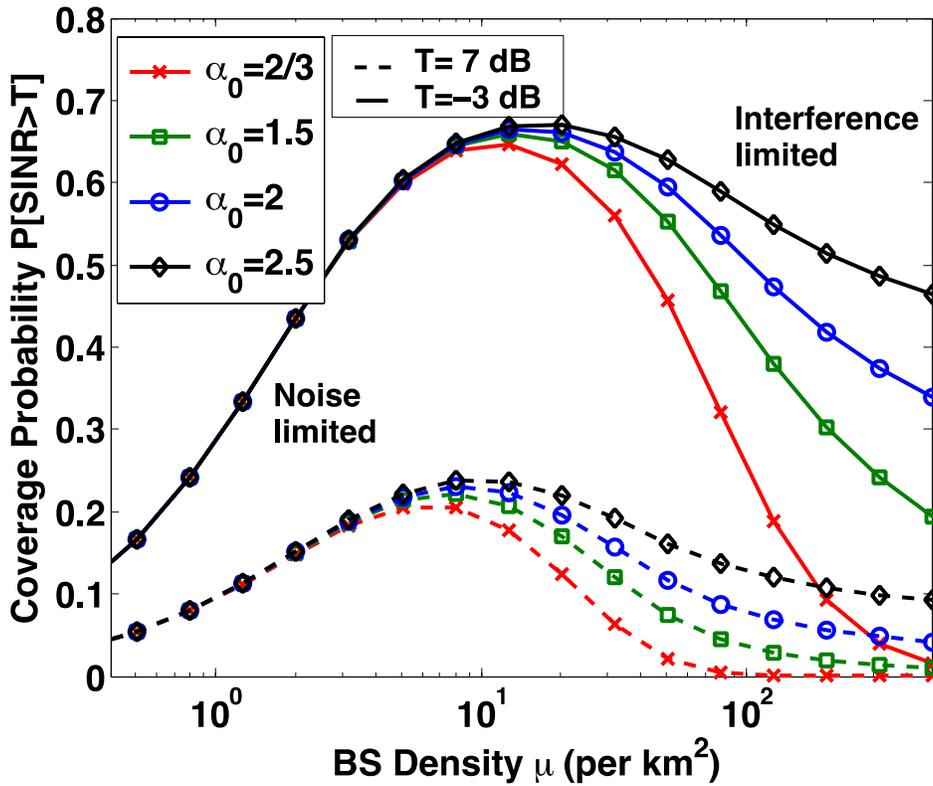
Figure 2: Probability of coverage vs. BS density (Poisson distributed, average per km<sup>2</sup>) in the 2D plane for SINR threshold  $T = 0.5$  (-3dB) and 5 (7 dB), close-in path loss exponent  $\alpha_0$ , and with  $R_c = 100$  m and  $\alpha_1 = 4$ . The noise is set in each case such that the SNR=20 dB at  $R_c$ . There is Rayleigh fading, but no shadowing or sectoring.
