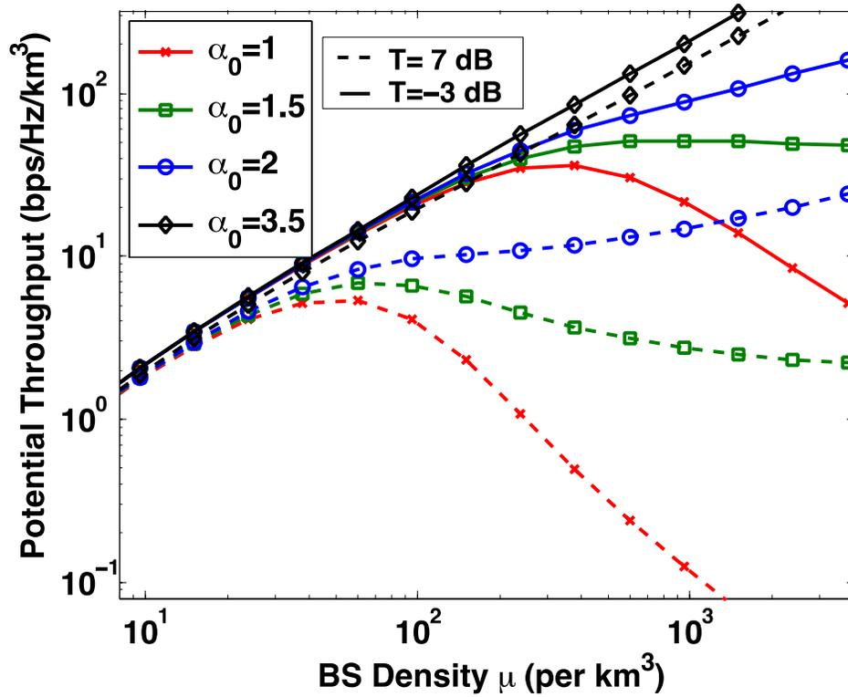
Figure 3: Potential throughput vs. BS density for 2D (top) and 3D (bottom) network topologies. Parameters are the same as for Fig. 2.
