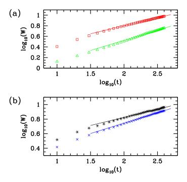
FIG. 9. (Color online) Global roughness as a function of time and corresponding least squares fits (solid lines) for: (a)  $\epsilon = 0.01$ , R = 10 (red squares; slope 0.30) and  $R = 10^3$  (green triangles; slope 0.38); (b)  $\epsilon = 0.1$ , R = 10 (blue crosses; slope 0.29) and  $R = 10^3$  (black asterisks; slope 0.22).
