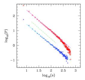
FIG. 7. (Color online) Pore size distribution (not normalized) above the transition point, for  $(R=10^3,\epsilon=0.125)$  (red triangles) and  $(R=10^3\epsilon=0.15)$  (blue crosses). The linear fits (solid lines) have slopes -1.43 and -1.37, respectively. The dashed line has slope -1.45.
