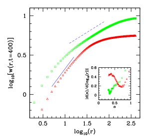
FIG. 10. (Color online) Local roughness of deposits grown with  $R=10^3$  and  $\epsilon=0.01$  (red triangles) and  $\epsilon=0.1$  (green squares). Solid and dashed lines are drawn to guide the eye and have slopes 0.75 and 0.35, respectively. Inset:  $|d\alpha/d\log r|$  as a function of  $\alpha$ , with symbols corresponding to the same parameters of the main plot.
