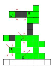
FIG. 1. (Color online) Schematic representation of the growing layer: substrate sites are empty squares, mobile adatoms are colored (green) squares, and non-mobile adatoms are black squares. The allowed steps of five adatoms, labeled A to E, are indicated by red arrows.
