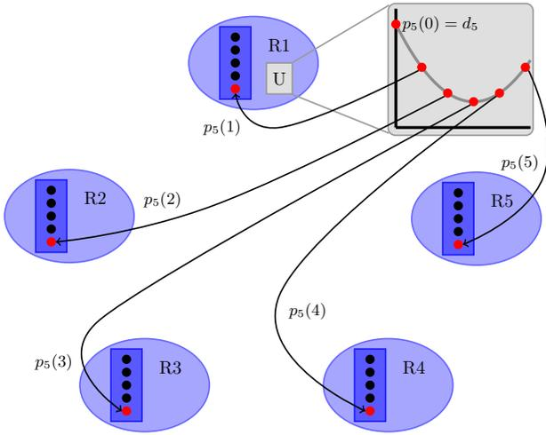
Fig. 2. An example of share distribution to securely store an entry in a distributed archive.
