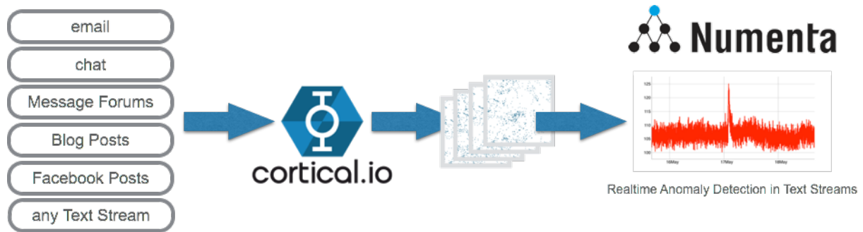
Fig. 20 Text Anomaly Detection using a HTM backend
