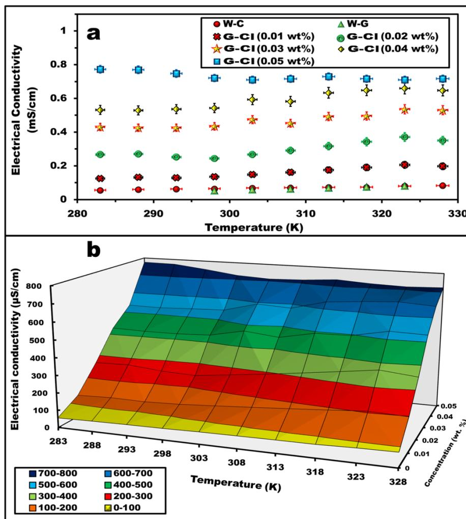
**FIGURE 5:** (a) Experimental observations of charge transport capabilities of G-CI based biocolloids with respect to bio-complex concentration and temperature of the colloid. (b) The full spectrum of electrical conductivity of the biocolloids with respect to concentration and temperature.
