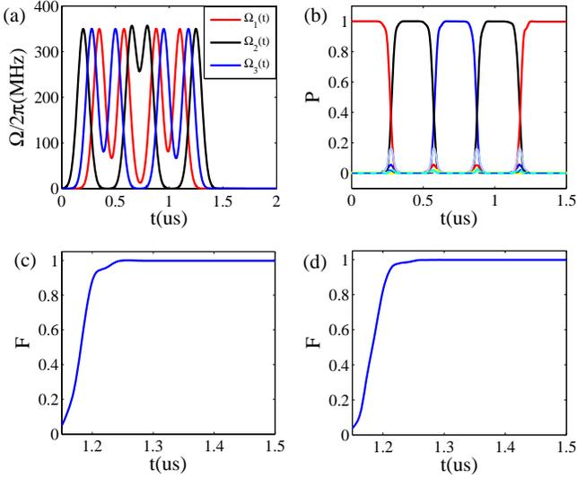
FIG. 3. **Numerical results for quantum state transfer from qubit 1 to 3 through 2 and then back to 1.** (a) The shape of the driven pulses. (b) Time evolution of the corresponding populations for the different quantum states, with  $g_1/2\pi = 200$  MHz. (c) The fidelity  $F$  versus time  $t$ , with  $\Delta g/2\pi = 0$ . (d) Fidelity  $F$  versus the time  $t$ , with the deviation  $\Delta g/2\pi = 40$  MHz ( $g_1/2\pi = 180$  MHz,  $g_2/2\pi = 200$  MHz,  $g_3/2\pi = 160$  MHz).
