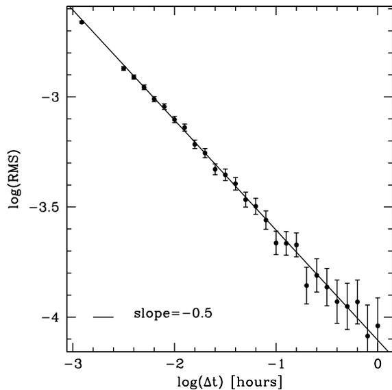
FIG. 6.— The RMS of the residuals of the individual data points from all of the light curves at various bin sizes in time. The weighted RMS of the unbinned data is 0.00221 as seen in the data point to the top left. We find that the RMS decreases as  $\sqrt{t}$  as expected in the photon-noise limited regime if the data points are uncorrelated. This decreases to 0.000276 when binned on 5 min intervals as shown in Figure 5.
