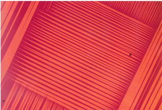
FIG. 2. Experimental martensitic microstructure. Different variants (colors)  $U_i$  can rotate via an  $\text{SO}(3)$  symmetry so as to joint together compatibly at twin boundaries. Courtesy of C. Chu and R. D. James [13].
