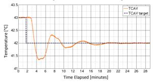
Figure 2: A 1-°C step change under the existing PI controller. The oscillations are due to water recirculation.
