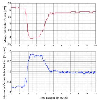
Figure 6: Measured flow control valve and heater actions.
