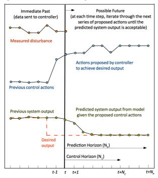
Figure 3: Basic concept of model predictive control.
