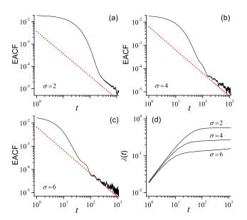
FIG. 2: (Color online) (a)-(c) The EACFs obtained by simulations (black solid lines) and by the hydrodynamics theory (red dotted lines). (d) The thermal conductivity calculated based on the EACFs obtained by simulations.
