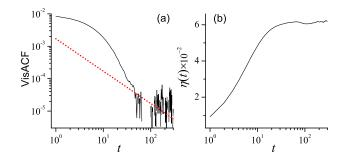
FIG. 3: (Color online) (a) The simulation result of the VisACF and (b) the corresponding sheer viscosity for  $\sigma = 4$ .
