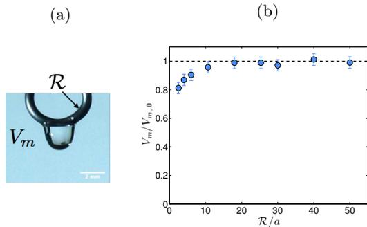
FIG. 2. (a) Picture of a silicone oil drop ( $V_m = 8$  mL,  $\eta = 10$  mPa  $\cdot$  s,  $\rho = 930$  kg/m<sup>3</sup> and  $\gamma = 23$  mN/m) placed on a curved fiber of radius  $b = 0.6$  mm and radius of curvature  $\mathcal{R} = 2.5$  mm. (b) Evolution of the ratio  $V_m/V_{m,0}$  as a function of the fiber normalized radius of curvature  $\mathcal{R}/a$  for a fiber of radius  $b = 0.6$  mm in the case of a perfectly wetting fluid (silicone oil on a steel fiber).
