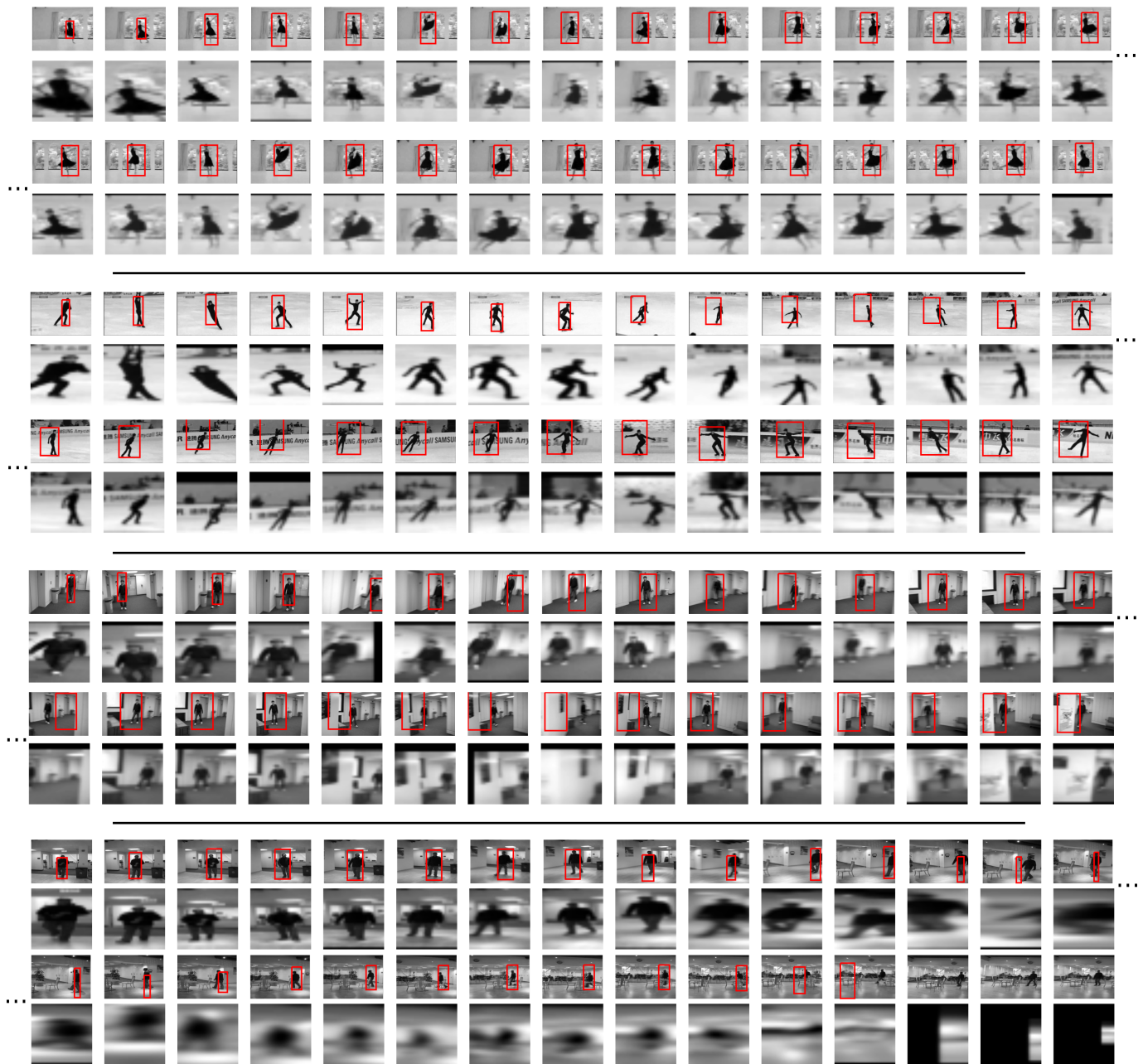
Fig. 14: Predictions of a KTH model on sequences from the TB-100 benchmark. From top to bottom we show the sequences Dancer , Skater2 , BlurBody and Human2 . To save space, we only show every seventh frame of the Dancer predictions and every tenth frame of the other sequences. The layout for each sequence is as follows: The first row shows 15 frames of one test sequence with a red rectangle indicating the location of the predicted glimpse. The second row contains the extracted glimpses. The third and fourth row show the continuation of the sequence.
