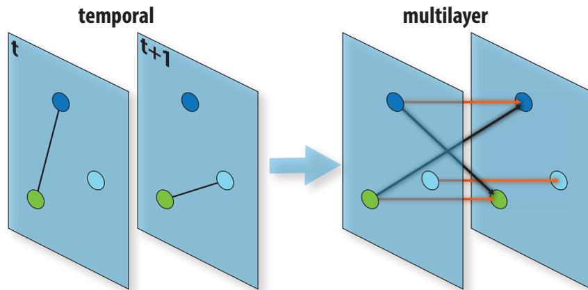
Figure 1: **Multi-layer representation of the temporal network.** We consider a temporal network of 3 nodes a 3 time steps (left). This network is mapped onto a multi-layer representation (right). Each node points to its future self (orange arrows), and to the future image of its present neighbors (black arrows).
