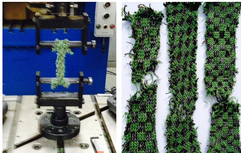
Fig. 1: View of the samples on the testing machine and after the stress test
