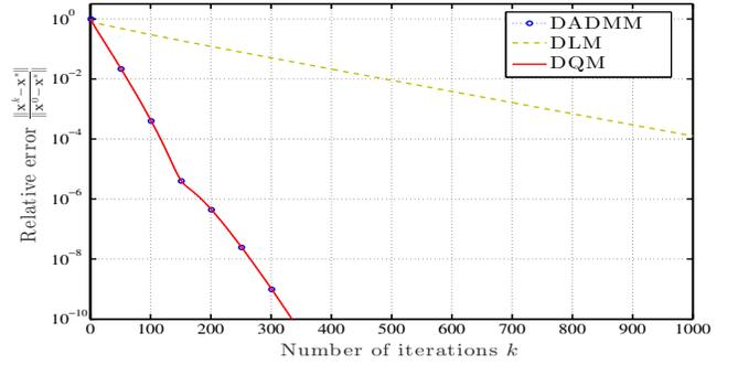
Fig. 1: Relative error  $\|\mathbf{x}^k - \mathbf{x}^*\| / \|\mathbf{x}^0 - \mathbf{x}^*\|$  of DADMM, DQM, and DLM versus number of iterations. The convergence path of DQM is almost identical to the one for DADMM, while DQM has less computation complexity. Further, DQM outperforms DLM in convergence speed by orders of magnitude, though at the cost of higher computation complexity.
