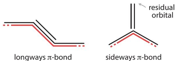
Figure S2: A path traveling longways (left) or sideways (right) through a double bond. Sideways traversal implies that the path is cross-conjugated. In the original graphical rules the residual orbital (not traversed by the path) must be covered by a (green) fixed point. Hence both methods predict destructive quantum interference for paths which traverse at least one  $\pi$ -bond sideways.
