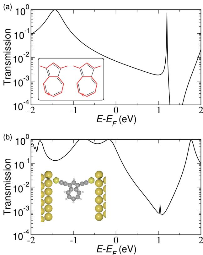
Figure 5: (a) Hückel transmission and (b) DFT transmission for Az-1,3. The inset in (a) shows the diagrams which do not contain an onsite-loop and shifts the interference feature away from the Fermi level. The same trend is observed in the DFT calculations in (b). Here the inset shows the geometry.
