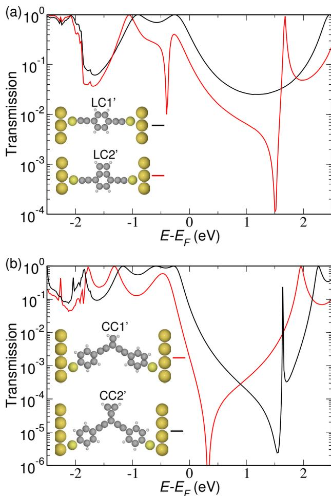
Figure 4: (a) Transmission calculated with DFT for the molecules LC1' and LC2' which are linked to gold using ethynyl-thiol groups. (b) Transmission for the molecules calculated with DFT for CC1' and CC2' which uses ethynyl-phenyl- thiol linker groups. The inset illustrates the geometry used in the calculations.
