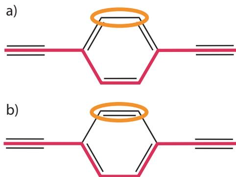
Figure S3: An alternative pair covering for a path traversing an even number of  $\pi$ -bonds in the sideways fashion. **a)** The drawn path is clearly cross-conjugated but the remaining atoms can be paired. **b)** When we redraw resonance structure a linearly conjugated path is evident.
