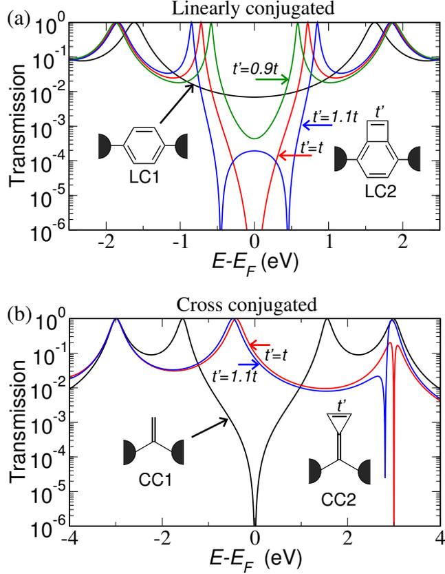
Figure 2: Transmission for a Hückel model with hopping  $t = -3$  eV between nearest neighbour atoms for pairs of (a) linearly-conjugated and (b) cross-conjugated molecules. The effect of bond length alternation is included by a modified hopping element  $t'$  for the bonds indicated in the insets.
