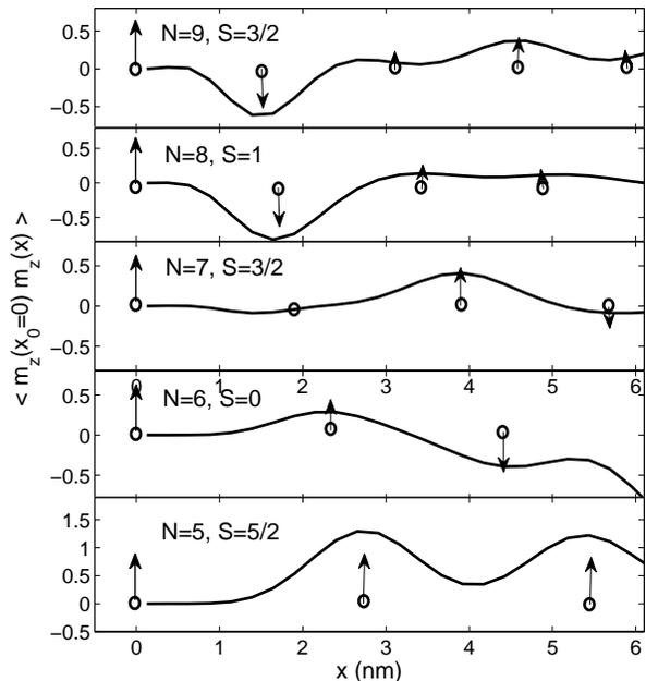
FIG. 4: Ground state spin-spin correlation function along the graphene edge for  $N = 9, 8, 7, 6$ , and  $5$ . The small circles with arrows represent the classical position of the localized electrons and their effective spin relative to the fixed electron at  $x = 0$ . As the density is lowered, the magnetic correlation between the nearest neighbors switches from antiferromagnetic coupling to ferromagnetic coupling. The vertical scale is kept the same in all the panels.
