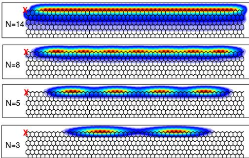
FIG. 1: Two-dimensional pair-correlation functions for  $N = 14, 8, 5,$  and  $3$  electrons occupying the zigzag graphene edge. The position of the fixed electron is indicated by a cross (red online). At  $N = 14$  charge oscillations only at the atomic level are observed. At lower  $N$  values,  $N - 1$  peaks arise and become increasingly localized, indicating the formation of an one-dimensional Wigner crystal.
