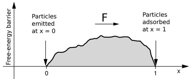
Figure 3. Sketch of the 1-D driven-diffusion model. Particles are emitted at the pore entrance  $x = 0$  and are adsorbed at the pore exit ( $x = 1$ ). Translocation requires the overcoming of the free-energy barrier with the help of an external force  $F$  acting along the  $x$  direction.
