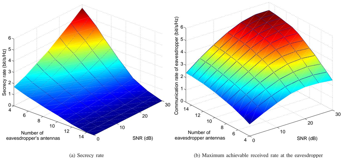
Fig. 5: The variation of the secrecy rate and the maximum achievable received rate between a legitimate transmitter and the eavesdropper when the proposed MT-MSE algorithm is invoked, where we have  $M = 4$  and  $\varepsilon_k = 1.5$ .
