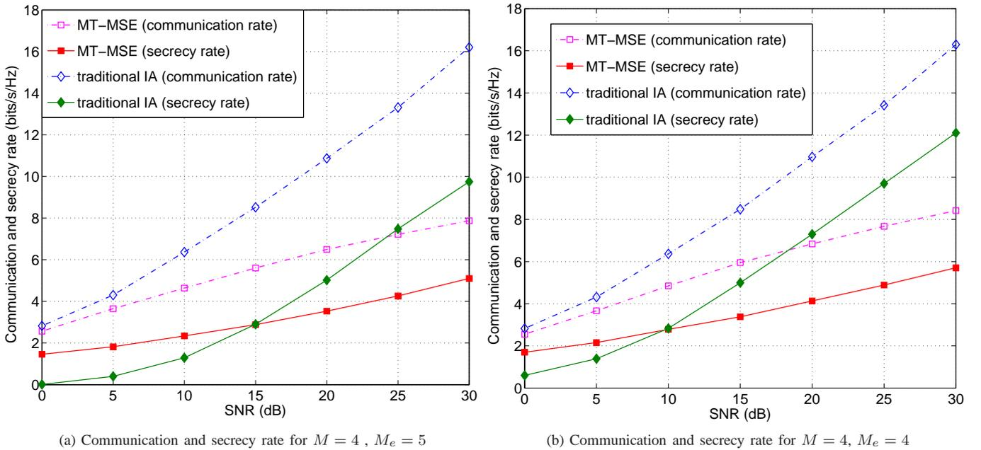
Fig. 4: Communication rate and secrecy rate versus SNR performance comparison of the proposed MT-MSE algorithm and the traditional IA algorithm [33], [49] in the presence of an “unsophisticated eavesdropper”, where we have  $M = 4$  and  $\varepsilon_k = 1.5$ .
