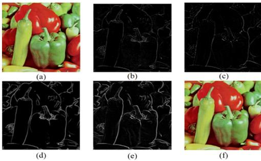
Fig. 3 A sample input image, its various edge-detected versions, and the final stego image. (a) Input image peppers, (b) image with edges detected by Laplacian edge detector, (c) Laplacian of Gaussian (LOG) edge detector result, (d) Fuzzy edge detector result, (e) Hybrid edge detector, resulted by combining (b), (c), and (d) images, and (f) final pepper stego image with embedded semantic information.
