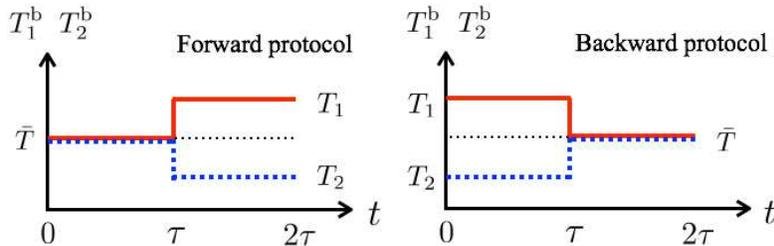
FIG. 2: Pair of protocols for estimating  $\Delta S_{\text{neq}}$  by utilizing (8). The heat baths  $T_1^b$  and  $T_2^b$  are changed in a stepwise manner, as indicated by the red solid and blue dotted lines, respectively. The forward and backward protocols are exactly time-reversed. The period  $\tau$  is set to be much longer than the typical relaxation time.
