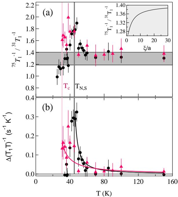
FIG. 2. (a) Ratio of the spin lattice relaxation rates of As to P ( ${}^{75}\text{T}_1^{-1}/{}^{31}\text{T}_1^{-1}$ ) and (b)  $\Delta(T_1T)^{-1}$  vs. temperature for  $x = 0.26$  ( $\bullet$ ) and  $x = 0.33$  ( $\blacktriangle$ ). The gray horizontal region indicates the range of values for purely magnetic fluctuations. INSET: The theoretical ratio as a function of the antiferromagnetic correlation length,  $\xi$ . Solid lines in (b) are best fits as discussed in the text.
