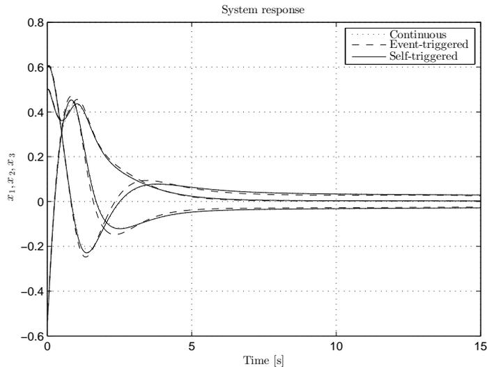
Figure 4: System response with  $w = 0$ .
