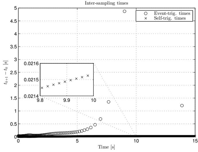
Figure 5: Inter-sampling times with  $w = 0$ .
