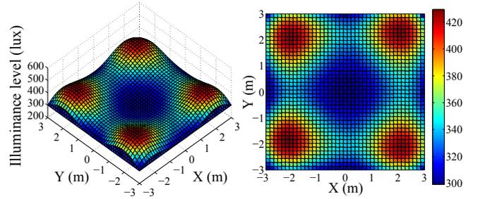
Fig. 12. A sample distribution of illuminance created by our proposed algorithm with the entire horizontal space illumination constraints
