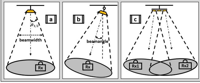
Fig. 2. Three different configurations: a) fixed beamangle and beamwidth; b) mechanically adjustable beamangle and beamwidth; c) electronically selectable beamangle and beamwidth
