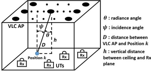
Fig. 1. System model for multi-user VLC indoor network
