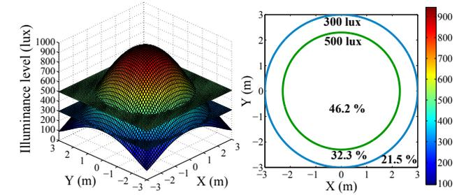
Fig. 13. A sample distribution of illuminance under the VICO framework
