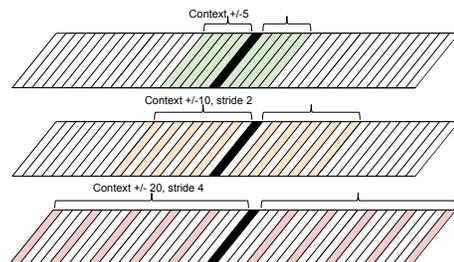
**Fig. 2.** Multi-scale feature maps with context  $\pm 5$  and strides  $\{1,2,4\}$  (3S/5). The final size of each feature map along the time dimension is 11. The three  $11 \times 40$  input feature maps are stacked as input to the CNN, similar to how RGB channels form 3 input feature maps in an image.
