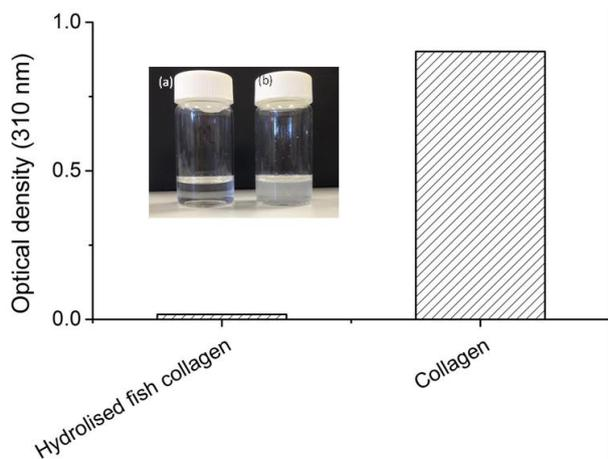
**Fig. S2.** Optical density of dissolved hydrolysed fish collagen and in-house extracted collagen. In inset optical image of 0.25% (w/v) of (a) hydrolyzed fish collagen and (b) collagen in 17.4 mM acetic acid solution. Both the graph and the optical image are in correlation and showed much higher optical density of collagen, thereby indicating that the collagen is present as a triple helix in the collagen suspension.
