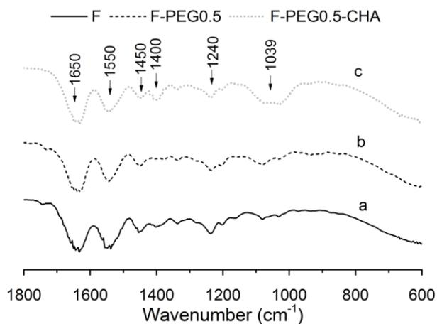
**Fig. 8.** ATR-FT-IR spectra of samples (a) F, (b) F-PEG0.5, and (c) F-PEG0.5-CHA. FTIR spectra (a) and (b) show characteristic peaks at 1650, 1550 and 1240  $\text{cm}^{-1}$ , attributable to amide I, II and III, respectively. Additionally, FTIR spectra (c) exhibits two additional bands at 1039 and 1400  $\text{cm}^{-1}$ , which are attributed to phosphate and carbonate groups, respectively.
