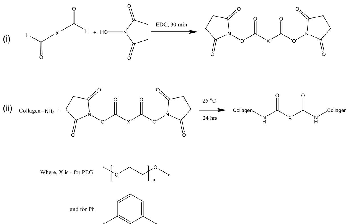
**Scheme 1.** Mechanism of the crosslinking reaction with varied diacid: (i) either PEG or Ph is NHS activated in presence of EDC, so that the crosslinking reaction of collagen can take place (ii). The functionalization of free amino terminations (mainly collagen lysines and amino termini) occurs through nucleophilic addition with activated carboxylic functions, leading to the formation of a covalent network of collagen triple helices.
