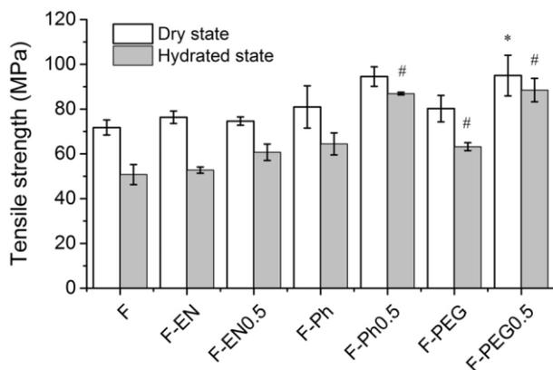
**Fig. S3.** Tensile strength of wet-spun and crosslinked fibres. ‘\*’ and ‘#’ indicate that mean values of corresponding crosslinked samples are significantly different from the wet-spun control group in dry and hydrated state, respectively ( $p < 0.05$ , t-test).
