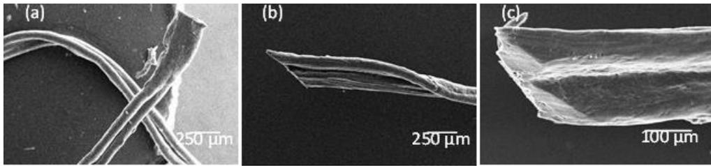
**Fig. S1.** SEM images of fibres wet-spun from collagen suspensions with 1.6% collagen (w/v) concentration showing surface striation (a) along the fibre and (b,c) at the fibre edges.
