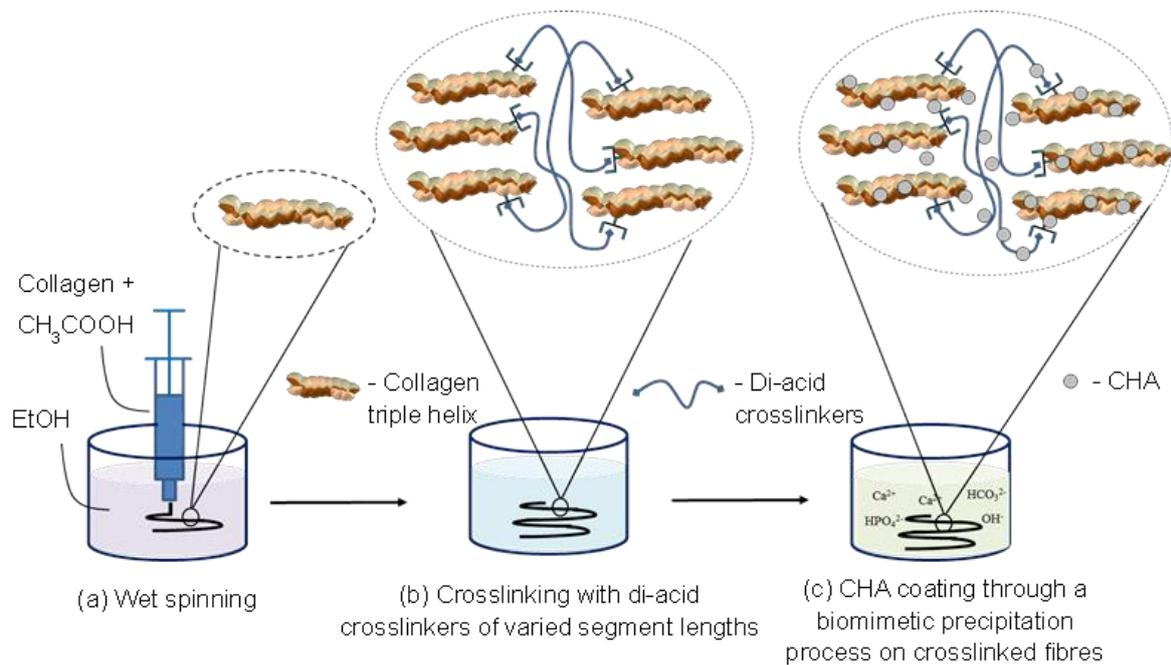
**Fig. 1.** Formation of biomimetic wet-stable fibres. (A) A suspension of collagen triple helices is wet-spun against ethanol, leading to the formation of micron-scale fibres. (B) Wet-spun fibres are reacted with varied diacids, resulting in a molecular network of covalently-crosslinked collagen triple helices. (C) Wet-stable covalently-crosslinked fibres are mineralised with CHA through a biomimetic process in order to obtain bone-mimicking fibrous systems.
