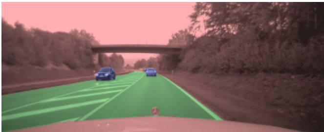
Fig. 8. Visualization of the final output of the classifier (best viewed in color). The grayscale input image has been tinted with the defragmented classification decisions. The information obtained facilitates an accurate representation of the scene in front of the vehicle.
