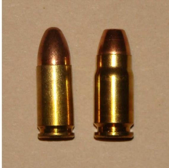
Figure 2: Loaded cartridges for the .357 SIG 125 FMJ (right) and the 9mm NATO 124 FMJ (left).
