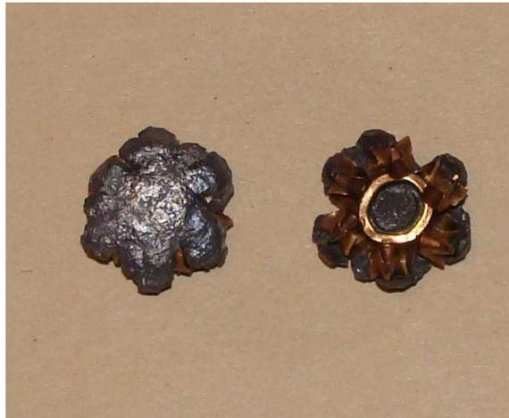
Figure 4: Front and back of expanded .357 SIG 125 SXT bullet after recovery from ballistic gelatin.
