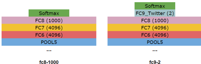
Figure 4: Architectures using the information contained in the original fc8 layer and weights. Configuration fc8-1000 reuses the whole architecture and weights from CaffeNet , while fc9-2 features an additional 2-neuron layer. The number between brackets next to fully connected layer makes reference to the amount of neurons they contain.
