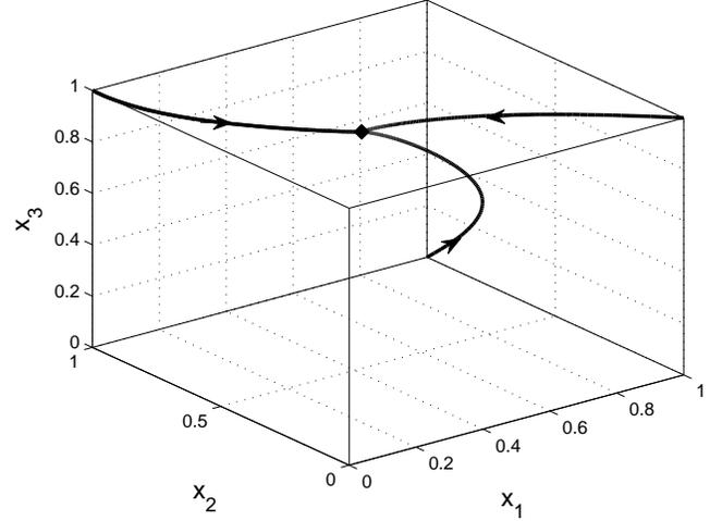
Fig. 2. Trajectories of (1) with  $n = 3$  for three different initial conditions in  $L_2$ :  $[1 \ 1 \ 0]'$ ,  $[1 \ 0 \ 1]'$ , and  $[0 \ 1 \ 1]'$ . The equilibrium point  $e_{L_2}$  is marked with a circle.
