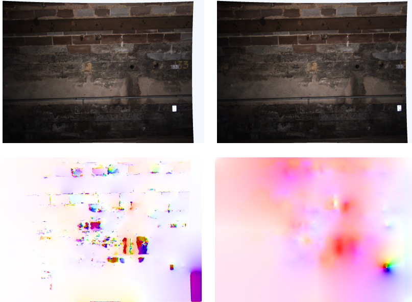
Figure 21: Up: Test case of the Wall sequence given by the Cerema. Bottom: Optical flow estimation obtained with (right) and without (left) treatment of the varying illumination. The images were divided in sixteen parts.
