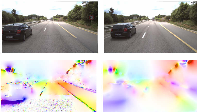
Figure 20: Up: Test case of the Highway sequence given by the Cerema. Bottom: Optical flow estimation obtained with (right) and without (left) treatment of the varying illumination. The images were divided in sixteen parts.
