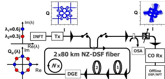
**Fig. 1:** Experimental setup: scatter plots of constellation symbols are shown at transmitter and receiver (after phase recovery) after 640 km transmission.
