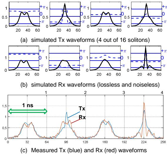
**Fig. 2:** (a) Four transmitted 2-Solitons: Solid lines show the absolute value and dashed lines show the phase. (b) The received solitons after 640 km over a lossless fiber. (c) The measured signals: back to back measurements (blue curves) and after 640 km NZ-DSF (red curves).
