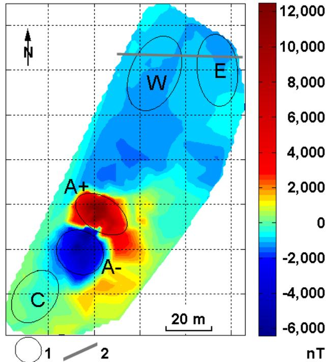
Fig. 2. Anomalous magnetic field within the study area. The normal magnetic field is 60,000 nT; sites (1), the local fault zone (2) (modified from Boyarskikh et al., 2012b).
