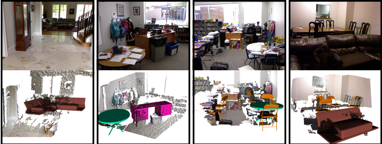
Figure 9. Qualitative pose and classification results on the NYUv2 dataset. Within each pair: Top: Original Scene; Bottom: Point-cloud with generic pose-aligned models inserted. Note that classification and pose-estimation are model independent. For visualization we used a random model per class.
