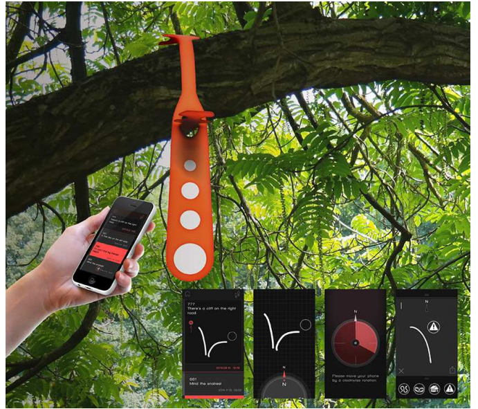
Fig. 3. LifeTie mobile sensing system - physical device and its mobile multimedia interface.
