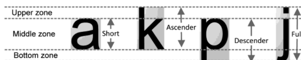
Figure 2: Illustration of the virtual lines and vertical zones in the text line.
