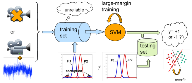
Fig. 1. Due to corruption in the training data the training and testing sample distributions are different from each other, which introduces errors into the decision boundary.
