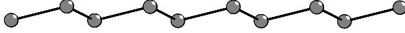
Figure 1. Sideview of the relaxed atomic structure of silicene. The structure is corrugated with out-of-plane corrugation of 0.57 Å.
