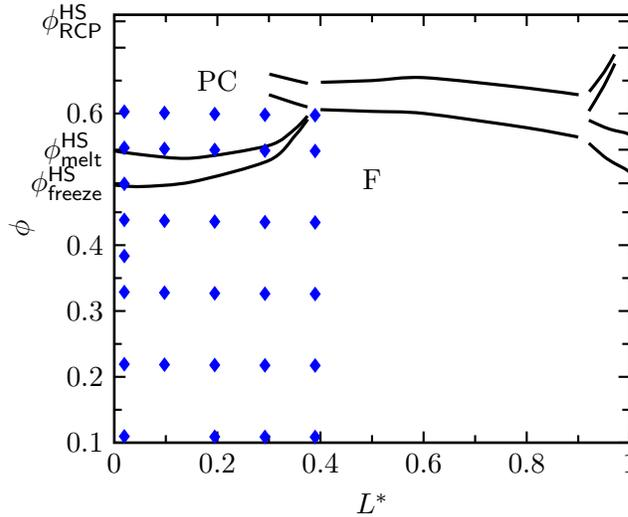
Figure 2. Schematic representation of the phase diagram of hard dumbbells [23]. We investigate systems in the fluid (F) and the plastic crystal (PC) phase. The filled diamonds ( $\blacklozenge$ ) indicate the state points investigated in this work, according to a Barker-Henderson mapping (2) of the site-site Yukawa pair potential (1) onto hard spheres.
