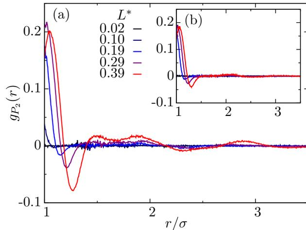
Figure 4. Orientational pair correlation function  $g_{P_2}(r)$  at a volume fraction  $\phi = 0.60$ : the black, blue, and purple curves present data for the systems in the plastic crystal (PC) phase and red in the fluid (F) phase, respectively. Inset: The same for a packing fraction  $\phi = 0.44$  where all systems are in the fluid phase.
