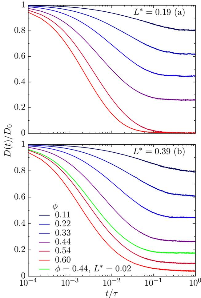
Figure 5. Time-dependent diffusion coefficient  $D(t)/D_0$  from the VACF at (a)  $L^* = 0.19$  and (b)  $L^* = 0.39$  for different packing fractions. The dashed line in (b) is at state point  $\phi = 0.44, L^* = 0.02$  for a direct comparison.
