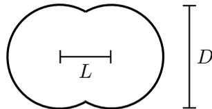
Figure 1. Sketch of the dumbbell geometry with dimensionless aspect ratio  $L^* = L/D$ .
