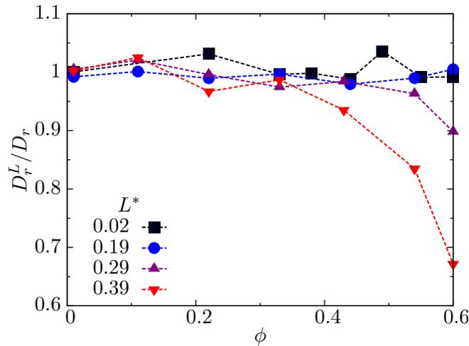
Figure 7. Dependence of rotational diffusion coefficients  $D_r^L$  at various elongations from exponential fits to DACF on volume fraction  $\phi$ . The statistical error of the data is estimated to be  $\pm 5\%$ , calculated from block averages over independent trajectories of length of  $10\tau$ .
