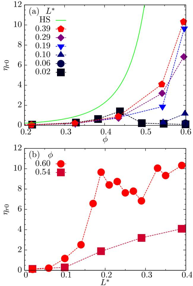
Figure 9. Steady shear relative viscosity difference  $\eta_{r0}$  (a) as a function of the volume fraction  $\phi$  and (b) versus elongation  $L^*$  at high densities. The hard sphere (HS) line (—) refers to the phenomenological Krieger-Dougherty theory [28, 38].
