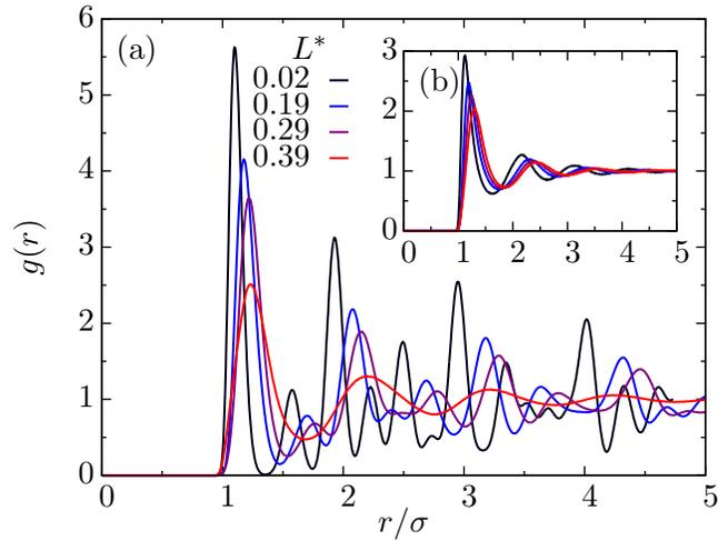
Figure 3. The radial distribution function  $g(r)$  for the dumbbell center-of-mass at a volume fraction  $\phi = 0.60$ : black, blue, and purple are in the PC, and red in the F phases, respectively. Inset: The same for a packing fraction  $\phi = 0.44$ , where all systems are in the F phase.
