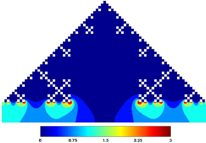
FIG. 12: Spatial dependence of the entropy production for the fourth fractal generation. It is shown the case of mild diffusion with  $c_2 = 0.9$  and distance between the electrodes  $L_y = 0.3$ . (Computer units.)
