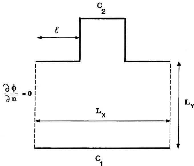
FIG. 1: Schematic representation of the diffusion cell for the first fractal iteration of a fractal generator. The dimensions of the cell,  $L_x = 3l$  and  $L_y = 2l$ , as well as the boundary conditions are indicated. For this fractal  $D_F = \frac{\log 5}{\log 3}$ .
