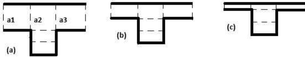
FIG. 3: Schematic representation of the diffusion cell for the first fractal iteration of a fractal generator. The distance  $L_y = ml$  (here  $l = 1$ ) is successively reduced from left to right: a)  $L_y = m = 0.3$  to b)  $L_y = m = 0.1$  and c)  $L_y = m \rightarrow 0$ .
