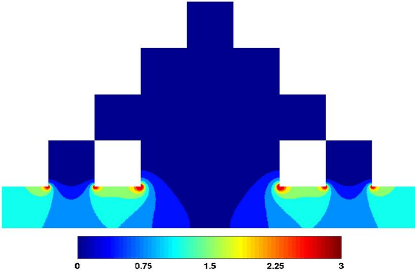
FIG. 8: Spatial dependence of the entropy production for the second fractal iteration. It is shown the case of mild diffusion with  $c_2 = 0.9$ , while the distance between the electrodes is  $L_y = 0.3$ . (Computer units.)
