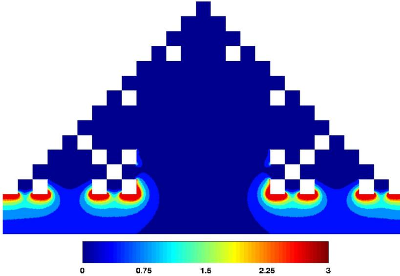
FIG. 9: Spatial dependence of the entropy production for the third fractal generation. It is shown the case of strong diffusion with  $c_2 = 0.1$ , while the distance between the electrodes is  $L_y = 0.3$ . (Computer units.)
