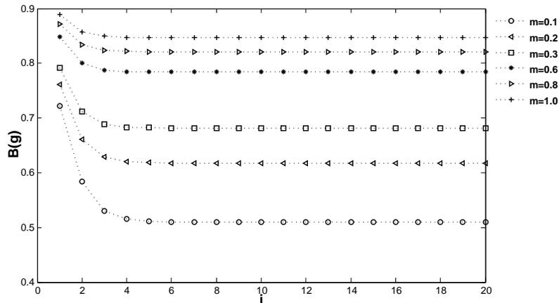
FIG. 4: Shown are the coefficients  $B(g)$  (eq.(16)) versus the fractal iteration  $i$  for various inter-electrode ( $m$ ) distances. We observe a saturation after the sixth fractal generation for a range of different distances.
