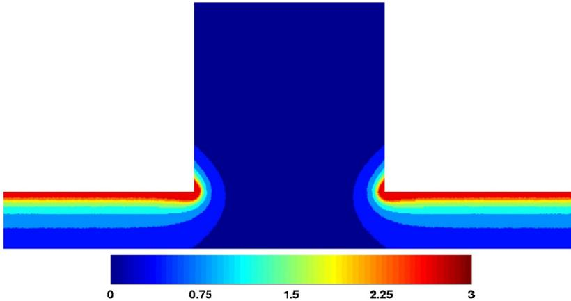
FIG. 5: Spatial dependence of the entropy production for the diffusion cell of Figure 1. It is shown the case of strong diffusion with  $c_2 = 0.1$ , while the distance between the electrodes is  $L_y = 0.3$ . (Computer units.)
