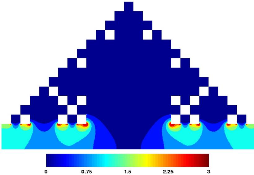
FIG. 10: Spatial dependence of the entropy production for the third fractal generation. It is shown the case of mild diffusion with  $c_2 = 0.9$ , while the distance between the electrodes is  $L_y = 0.3$ . (Computer units.)
