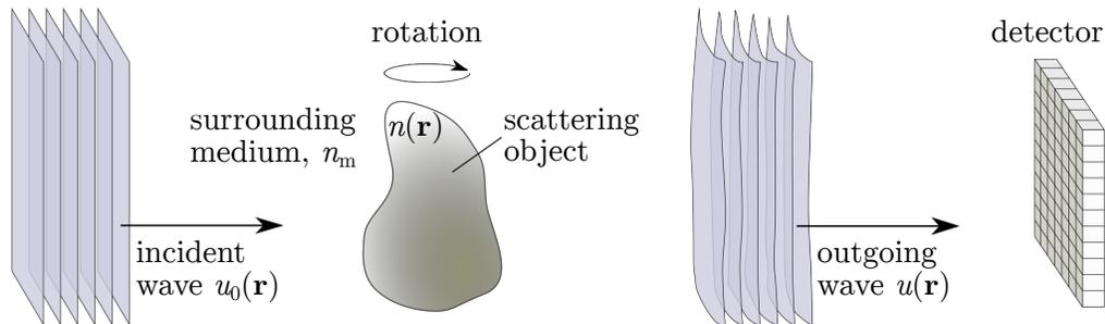
**Figure 1, Tomographic data acquisition.** An incident plane wave  $u_0(\mathbf{r})$  is scattered by a transparent object with the refractive index distribution  $n(\mathbf{r})$ . A detector collects the scattered wave  $u(\mathbf{r})$ . Multi-angular acquisition is facilitated by rotation of the sample.
