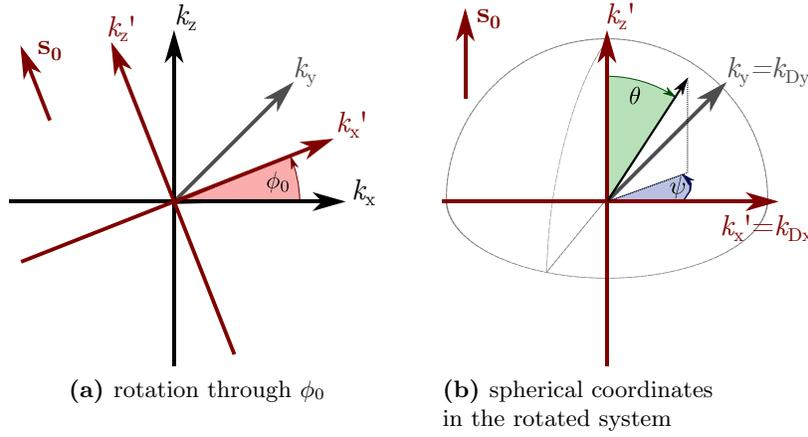
**Figure 5.3, Coordinate transforms for 3D backpropagation.** **a)** The coordinate system of the detector (red) is rotated about the  $y$ -axis which corresponds to a rotation about the  $k_y$ -axis in Fourier space. **b)** The position on the semi-spherical surface with the radius  $k_m$  is described in a spherical coordinate system with the polar angle  $\theta$  and the azimuthal angle  $\psi$ .
