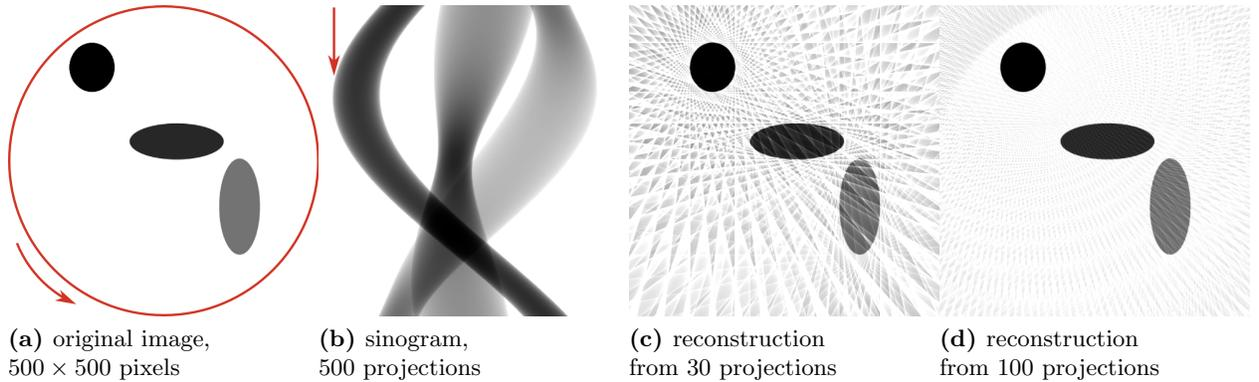
**Figure 1.2, Backprojection.** a) The original two-dimensional image contains ellipses of different gray-scale levels. b) The sinogram shows 500 projection of image (a) from  $0^\circ$  to  $180^\circ$ . For the computation of the sinogram, only the circular region of the original image (red) was used. c) Reconstruction using 30 equidistant projections. d) Reconstruction with 100 projections. The sinogram and reconstructions were created with the Python library radon [12].
