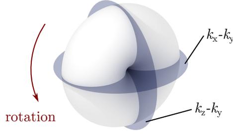
**Figure 5.2, Horn torus.** As a result of the Fourier diffraction theorem, images acquired perpendicularly to the sample-rotating axis ( $y$ ) fill a horn torus-like shape in Fourier space. The resulting reconstruction exhibits missing angle artifacts, as shown in figures 5.4 and 5.5
